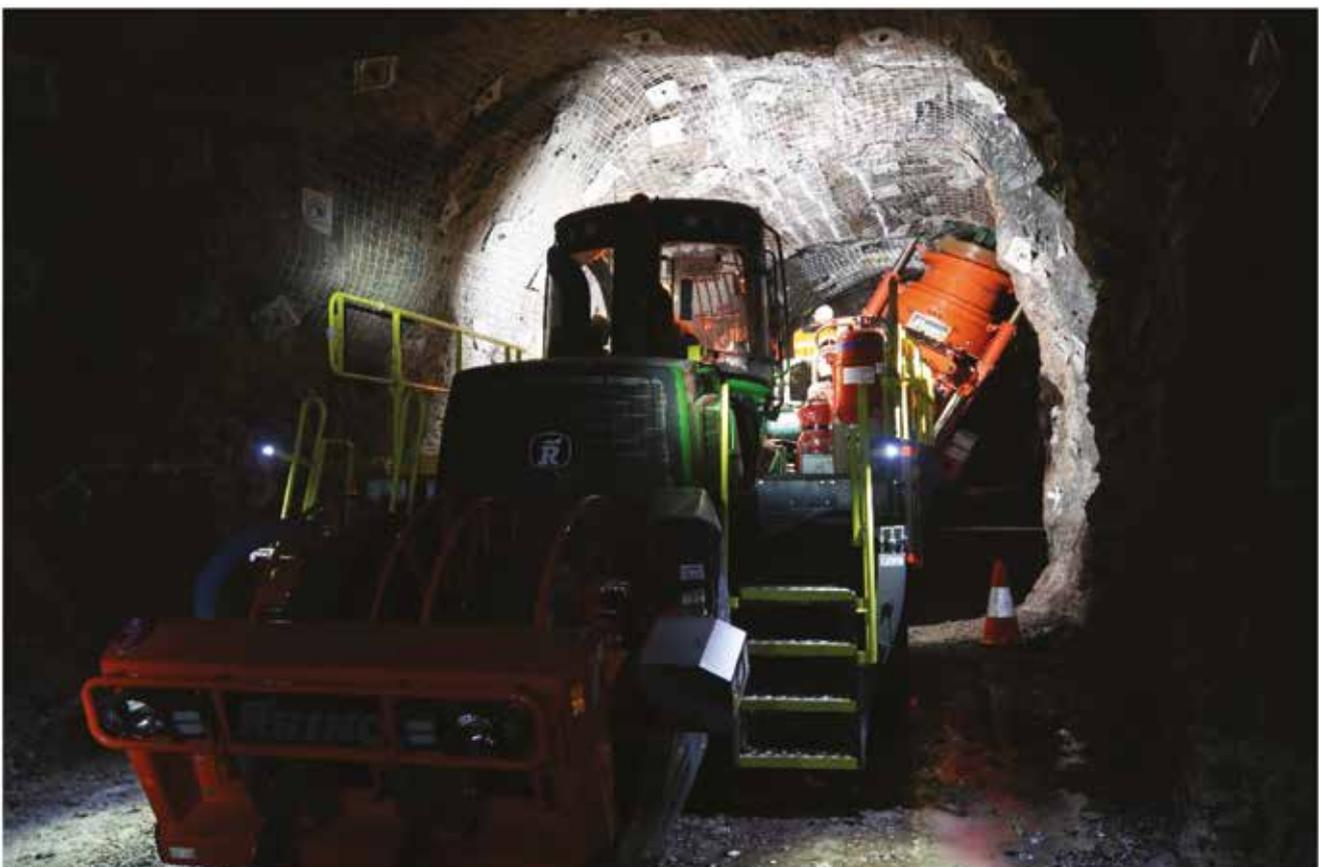
Figure 4. Mobile Rhino 100 raise boring system operated by a single operator.
